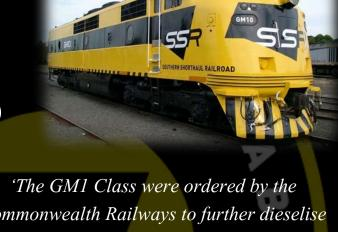
Commonwealth Railways to further dieselise the Railways. Based on an international design they had a local design variation to reduce axle loads by utilising a non-driven centre axle in each bogie via an A1A-A1A arrangement. This did however slightly reduce the tractive effort by removing weight from the driven axles.'
